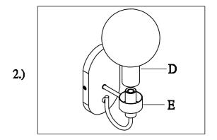
Step.2:Put the glass(D) into socket(F)
