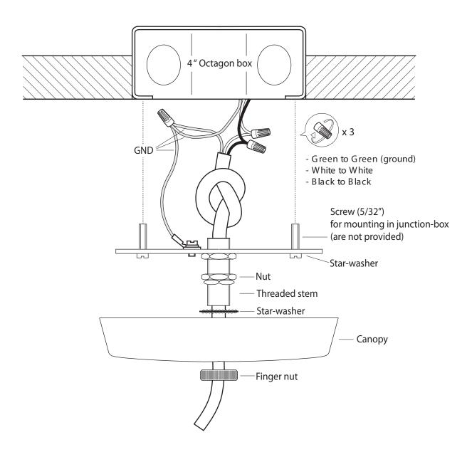
1 Thread the wire 3x18 AWG cord through finger nut, canopy threaded stem with nut and star-washer
