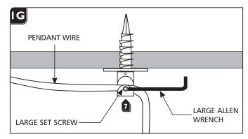
D Hook the fixture pendant wire into the swag hook and secure it in place by tightening the large set screw.
