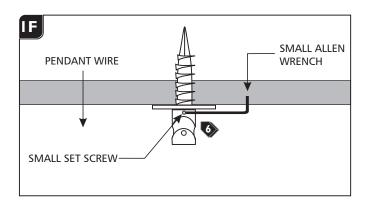
Secure the swag hook to the threaded washer by tightening the small set screw.
