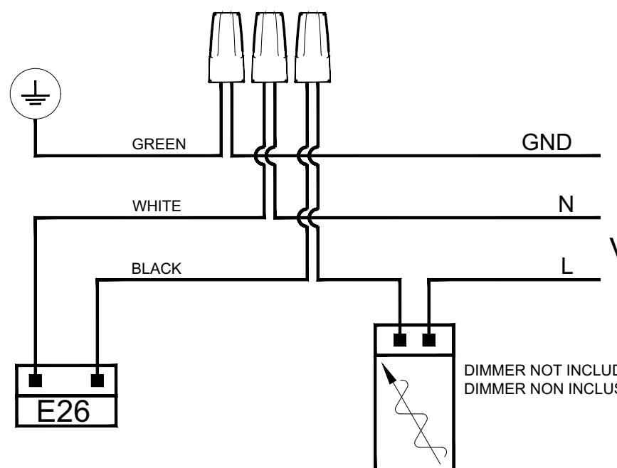
Dimmable wiring diagram (TRAILING EDGE - LEADING EDGE)
