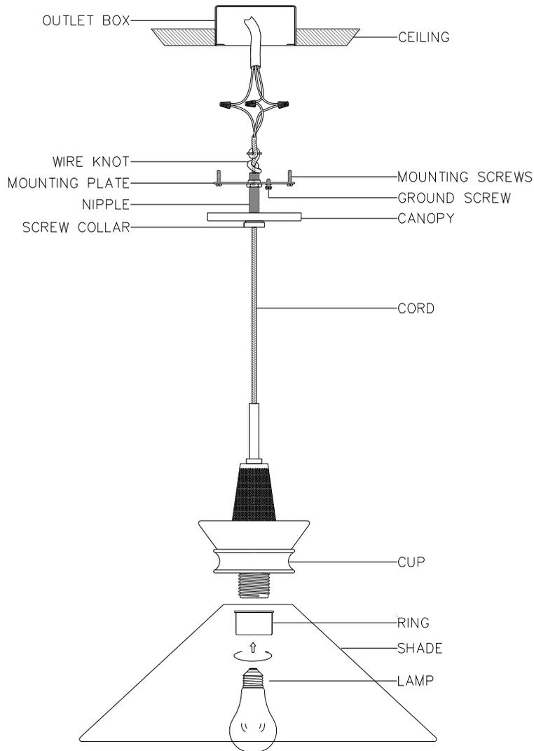
**WIRE NUT/TAPING DIAGRAM**
