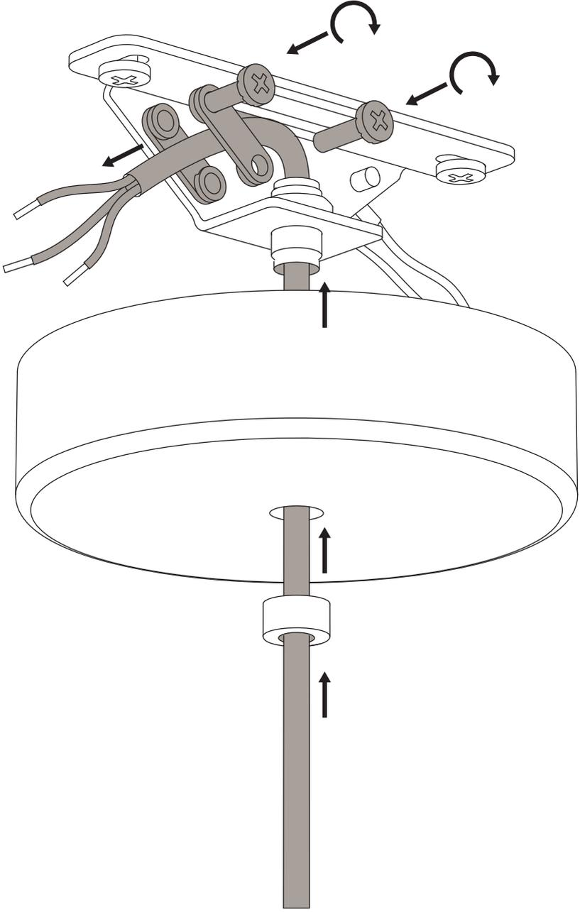
To inspect the electrical connections, remove the canopy enclosure by unscrewing the strain-relief located below it.
