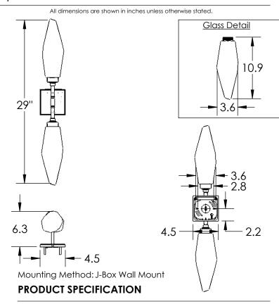
Construction: Aluminum Body, Blown Glass
