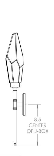
\*\*NOTE\*\* DRIVER TO BE INSTALLED IN JUNCTION BOX. MINIMUM SIZE J-BOX REQUIRED IS 4" L X 4" W X 1.5" D
