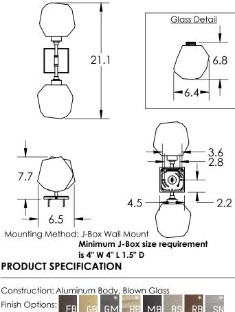
Construction: Aluminum Body, Blown Glass Finish Options: MB B GB GM Glass Options: CS BG Suspension Method: Wall Mount Weight(lbs.): 8LBS UL Rating: Dry Top Diffuser: Closed Glass Bottom Diffuser: Closed Glass Light Source: DC LED Electrical Qty: 2 Wattage (Watts):6 Voltage (Volts): 120 V Source Lumens: 466 Dimming: Forward/Reverse Phase to 1% CCT: 2700K or 3000K Driver Quantity & Location: 1, in J-Box CRI: 93+ Power Factor: >0.9
