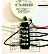
NOTE: The Grev and Purple wires are used for 0-10V dimming. If not applicable cap wires. Wires must be capped separately, or pendant will dim to zero.
