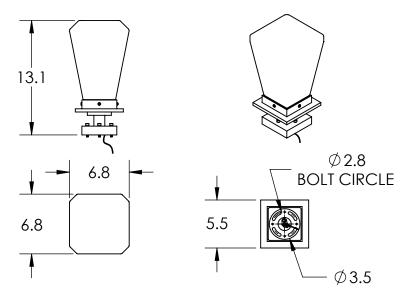
Mounting Method: Mounts Directly to Pier
