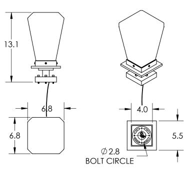
Mounting Method: Mounts Directly To Pier
