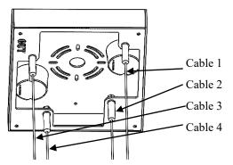
Set cable 1 at the height you want the fixture at, then size the rest of the cables based on the offset from the table.
