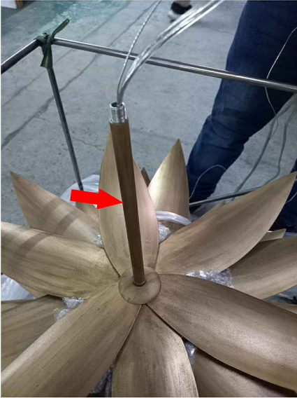
10. THREAD THE STEM INTO FIXTURE
