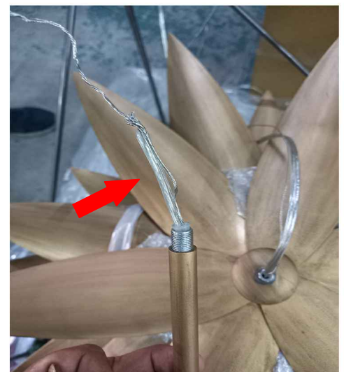
9. SLIP WIRE OVER THE STEM
