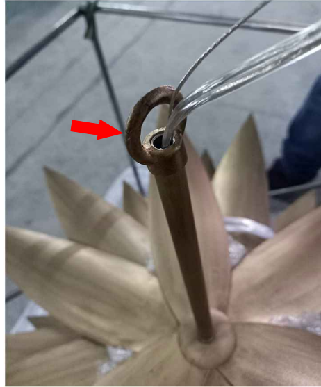
11. THREAD THE LOOP INTO STEM
