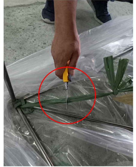
12. CUT THE REST OF PLASTIC TWINE
