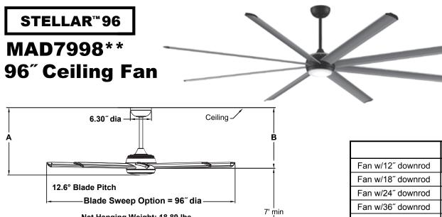
Net Hanging Weight: 18.89 lbs (Motor Assembly Only) MAD7998 W/B7998-96 Net Hanging Weight: 35.27 lbs Floor
