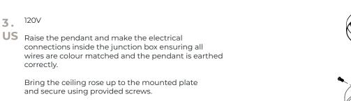
Note: Ensure that the weight of the pendant is fully supported during the electrical installation.
