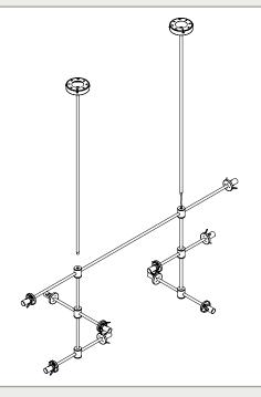
3 Raise the pendant and make the electrical connections ensuring all wires are colour matched and the pendant is earthed correctly.
