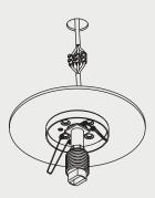
B. Before mounting the fitting, ensure that the surface being mounted to is flat and smooth to create a secure seal around the back plate.
