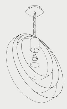
**4** Unscrew the bolt off the inner ring, bring the inner ring to the Lunar Medium body and screw into place securely
