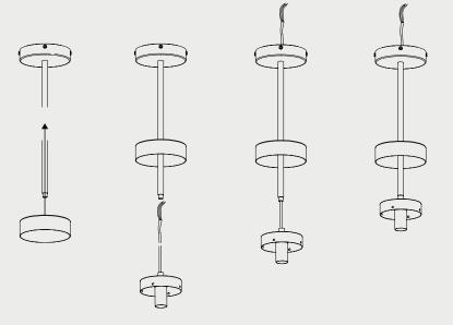
Raise the pendant and make the electrical connections ensuring all wires are colour matched and the pendant is earthed correctly.
