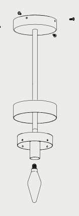
5. Raise the shade to the lamp-holder and fit the bulb through the hole on the top of the shades.
