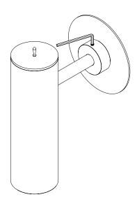
When the screw has been removed, slide the collar along the shroud to show the two holes on the back plate.
