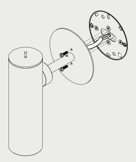
**5**. With the fitting securely fixed to the wall, slide the collar back into place along the shroud and replace and fully tighten the small screw to lock the collar into place.
