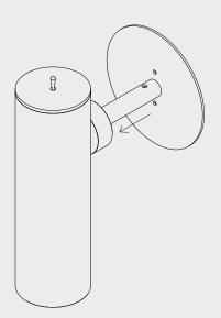
**4**. Bring the fitting to the wall and make the electrical connections.
