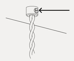
With the ceiling box securely fixed to the mounting plate, raise each pendant to access the lampholder.
