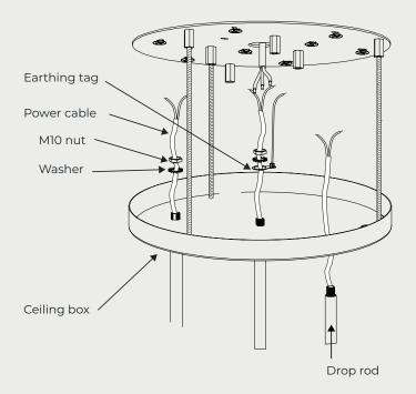
**5** Make all required electrical connections between the pendants within the ceiling rose cover.
