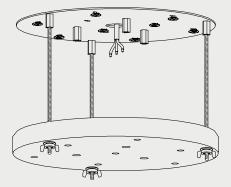
**3.** Thread the cable from the Artes Pendants through the drop rods and fix the two together using 4 x countersunk screws until are fully secure.
