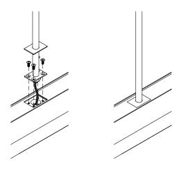
4. Feed the power cable from each drop rod into the ceiling rose cover through the hole, then use the washer and M10 nut to secure each Artes Pendant to the ceiling rose cover.
