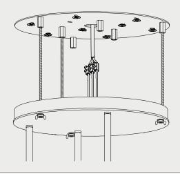
6. Make the electrical connections inside the ceiling rose cover ensuring all wires are colour matched and the pendant is earthed correctly.
