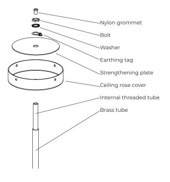
**1**. Thread the cable from the Artés Pendant through the drop rod and fix the two together using the 4 x steel countersunk screws until they are fully secure.
