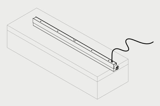
2. Bring the base up to the bottom of the Artés floor and secure with the 4 x supplied screws.
