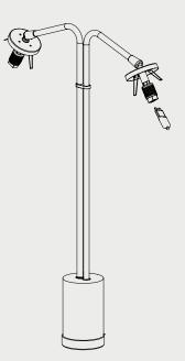
2. Pinch the spring clips inwards and hold, slowly feeding the opal glass shade over the spring clips. Do not release the opal glass shades too quickly.
