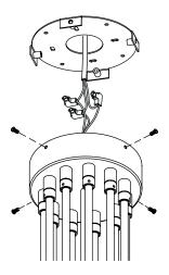
2. Fit the bulbs (not supplied) and shades to the pendant. Pinch the spring clips inwards and hold, slowly feeding the opal glass shade over the spring clips. Do not release the opal glass shades too quickly.
