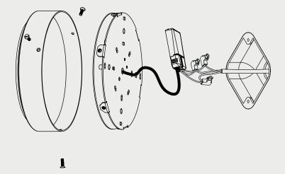
A. Make power connection to the LED driver. See wiring diagram.
