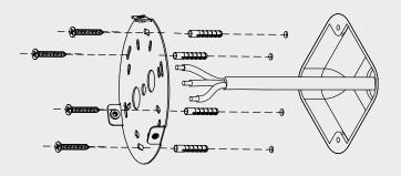
2. Bring the body of the light closer to the mounting plate and make the electrical connections within wall rose, ensuring all wires are colour matched and the pendant is earthed correctly.
