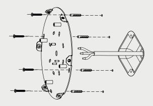
2. Bring the body of the light closer to the mounting plate and make the electrical connections within wall rose, ensuring all wires are colour matched and the pendant is earthed correctly.
