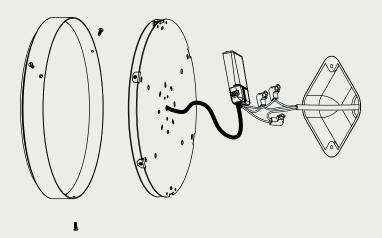
A. Make power connection to the LED driver. See wiring diagram.
