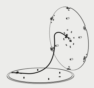
**3**. Fit the driver into the cavity of wall or ceiling.
