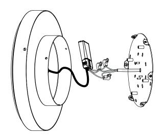
$\ensuremath{\mathsf{A}}.$  Make power connection to the LED driver. See wiring diagram.
