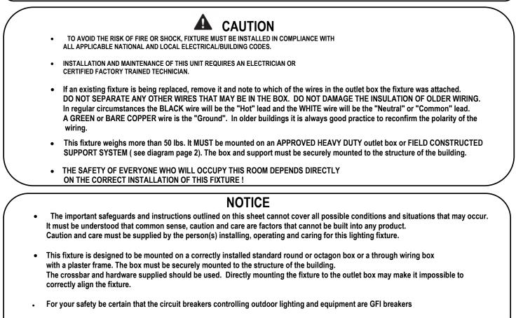
WITH MAXIMUM LAMPING THE FIXTURE WILL USE 960 WATTS! A standard 600 watt dimmer CANNOT BE USED. A 1000 WATT DIMMER MUST BE INSTALLED FIXTURE PREPARATION
