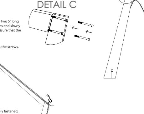
**4.** With the body components now securely fastened, press the wire and cord stock into the groove covering the joint.
