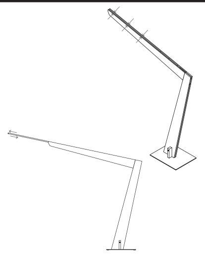
**9.** With the boom now set to the desired length, attach it using the two #8 wood screws.
