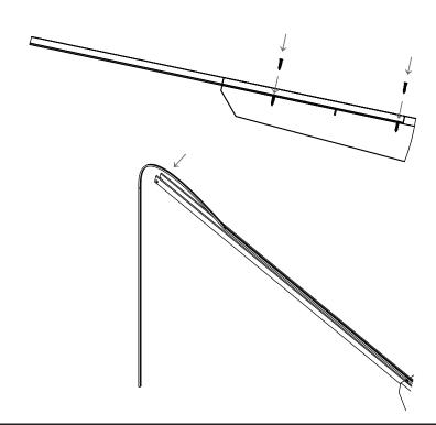
**10.** With the boom now fully assembled drape the cord over the roller at the end of boom arm
