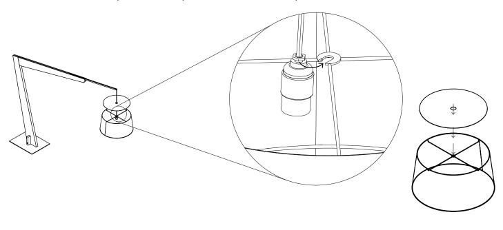
Following shade and top diffuser installation, install the bulb into the socket
