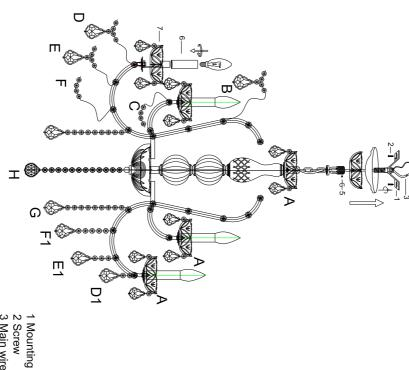
6 Iron Pipes 4 Junction pole 3 Main wire 7 Glass dish 5 Screw 2 Screw
