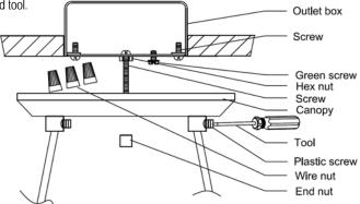
5. Fasten the white fixture lead wire to the white wire in the outlet box.
