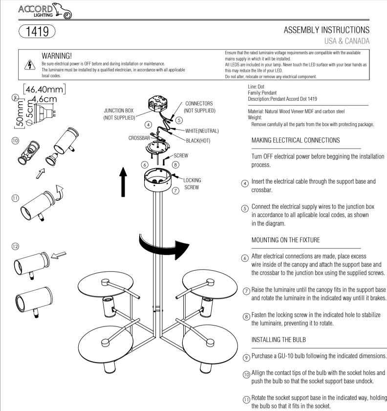
After the bulb is already connected to the socket, push the socket support base fitting it to the luminaire. With the socket support base docked to the luminaire, the bulb
