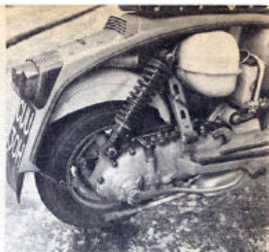
Under the other panel you'll find the "works". Oil filler, level and drain plugs, plus suspension unit are reached from this side
