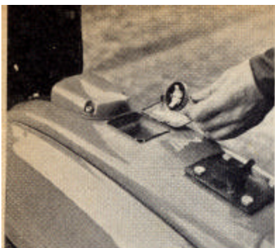
Fuel tank cap is tucked safely away under the hinged dual seat. 25:1 petrol mixture is used during and after running-in period
