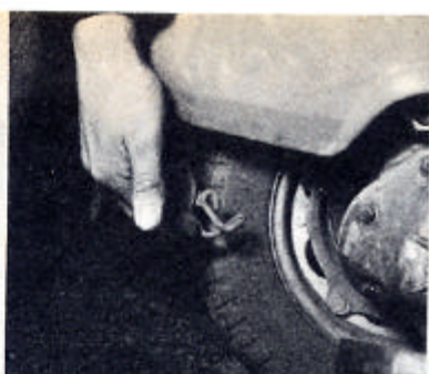
One of the new items on the Bertone-styled Grand Prix is the method of attaching side panels. It cleans up bodywork
