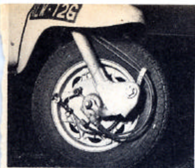
The front brake on the Grand Prix 150 is a single-leading shoe drum and could do with an improvement in stopping power
