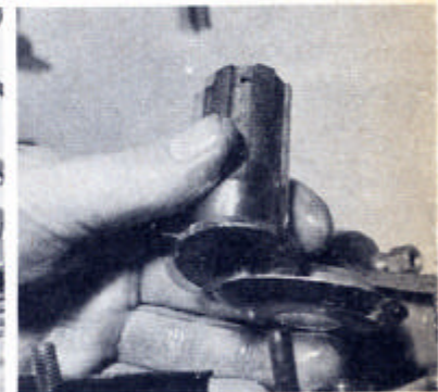
The shock absorber sleeve is splined and must have no wear on spline faces. Don't forget the baffle plate under shaft
