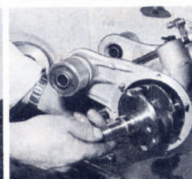
Turn crankshaft until the conrod is at its lowest position. It should then be easy to wobble the complete assembly from case
