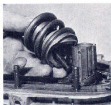
Knock down tab washer on clutch centre nut, lock motor and undo nut. The shock absorber nut can also be undone and the . . .
