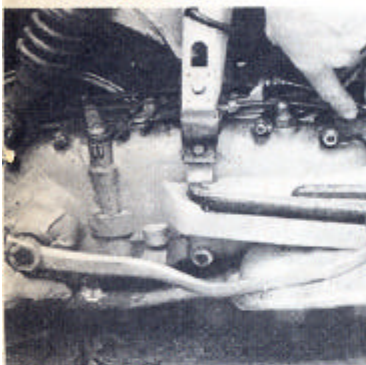
The exhausts tend to vibrate and fracture the two mounting brackets. Check both as shown, as a new exhaust system is expensive
