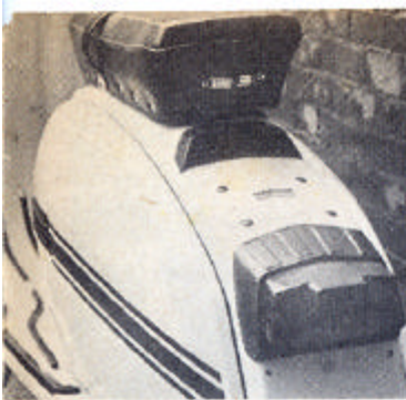
Another view showing the easy-to-clean lines. The whole rear lamp unit and the air outlet grille above are made of plastic material
