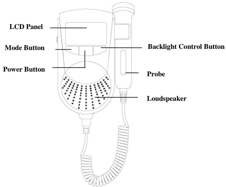
**Fig.3-1 Front Panel**
