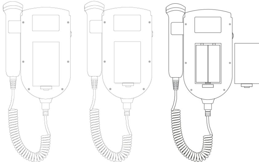
**Fig.4-2 Replacing Battery**
