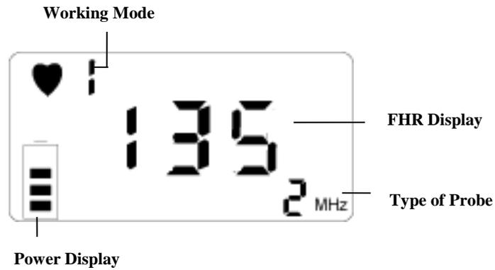
Fig.3-4 LCD Display
