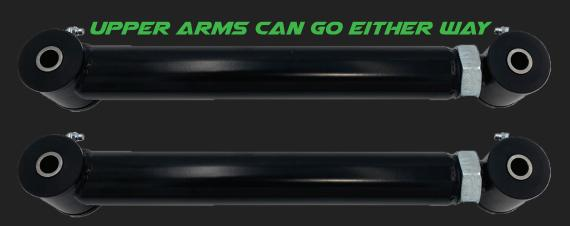
Measure from center to center of bolt holes.
