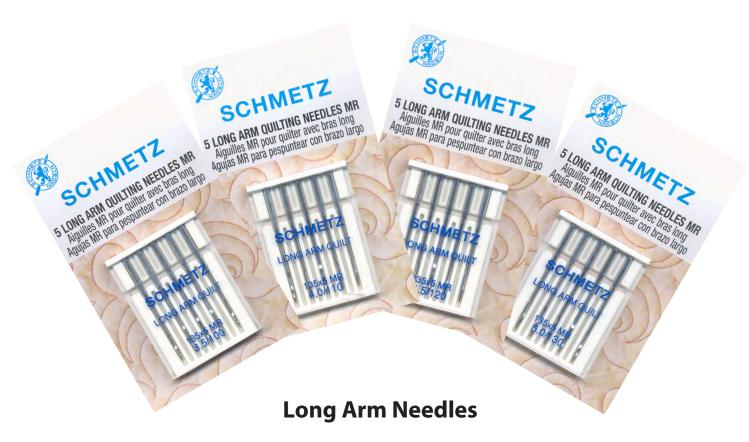
135x5 MR needles, the most popular needle system used by long arm quilting machines, are available in a five needle pack. This needle has a long groove and a scarf that is deep with the same cross section as the upper blade area. Using the correct needle system is essential for long arming, so check your owner's manual. Needle system 135x5 is also known as 134, 134R, 135x7, SY 1955, DPx7.
