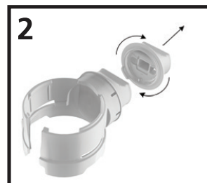
2 Separate the energy source (non-rechargeable lithium metal coin cell battery) from the collar and dispose in accordance with federal, state and local regulations.
