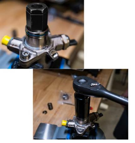
USING HIGH PRESSURE FUEL PUMP REMOVAL TOOL AND RATCHET REMOVE THE BASE SEAL
