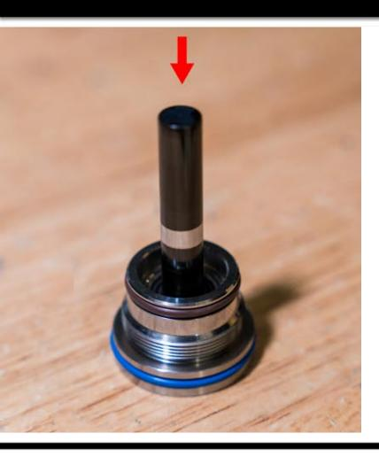
PUSH THE PISTON BACK INTO REPLACEMENT SEAL HOUSING
