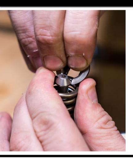
REINSTALL RETENTION CLIP UNDER TIP OF PISTON TO KEEP SPRING DEPRESSED
