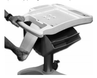
2. Using a Phillips screw driver, fasten the card reader assembly under the front handle, aligning it with the holes provided under the front handle.
