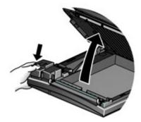
2. To set the tray for A4 paper, slide the paper guide toward the rear of the device.
