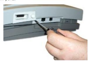
3. Grasp the side edges of the communications board and work it back and forth in the slot as you pull it out along its rails.
