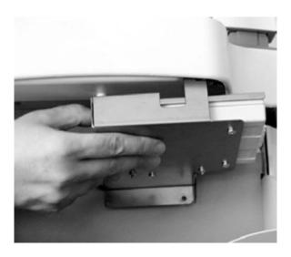
3. Tighten the three mounting screws to secure the modem to the trolley.
