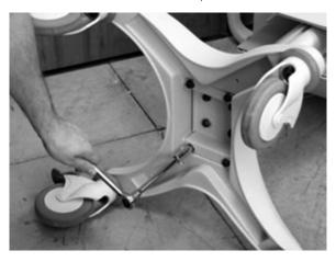
2. Remove the remaining bolts and mounting plate.
