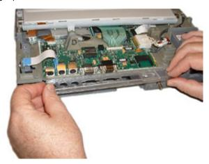
6. Rotate the bezel to the upright position as shown in the following photograph.
