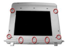
4. Gently flip over the display assembly, so the LCD panel is face down, and remove the display cover.
