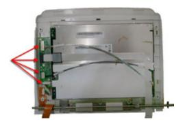
6. Gently lift the LVDS board from the display assembly and clean any remaining adhesive (1) from the plastic bezel.
