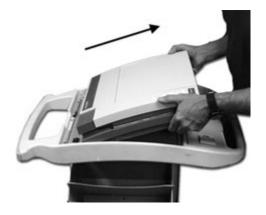
3. Lift the device from the trolley.
