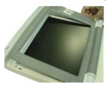
Reattach the display assembly to the device.
