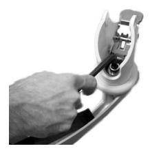
5. Install the replacement caster on the trolley.
