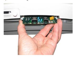
4. Insert the new communications board, sliding it onto the rails until it is seated in place.
