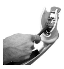
6. Install the wheel and attach it with the wheel bearing shaft and nut.
