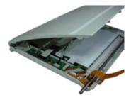
8. Gently flip over the assembly so the LCD is facing up and reattach the ten screws that secure the assembly to the display cover.
