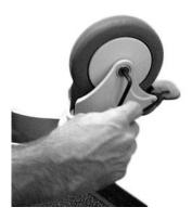
4. Using an Allen wrench, remove the bolt holding the caster to the trolley.
