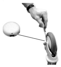
3. Using an Allen wrench, remove the wheel shaft and wheel from the caster.
