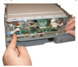
7. With the new bezel in place, replace the top cover by reversing the steps described previously.
