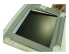
Reattach the display assembly to the device.
