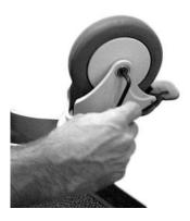
7. Using a small mallet, tap the bearing dust covers back in place.
