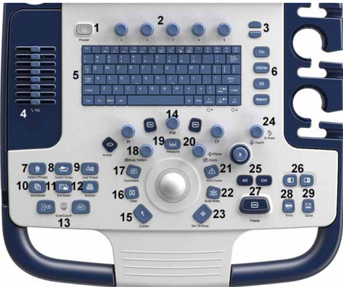
Figure 4-5 Control Panel Tour
