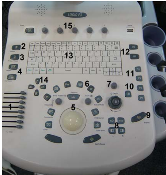
Figure 4-5 Control Panel Tour
