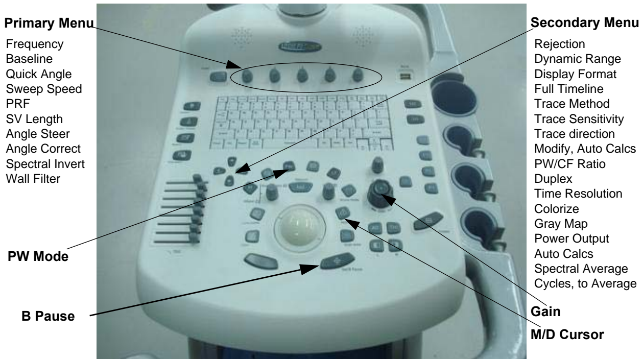
Figure 4-14 Controls available in Doppler Mode
