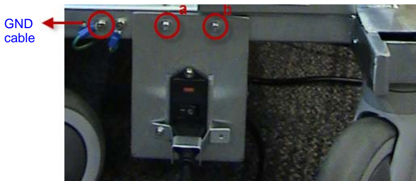
Figure 8-86 Removing Transformer Assembly
