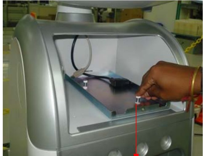
Using two Captive fastener mount VGP Tray bottom to the Sytem Utility box.
