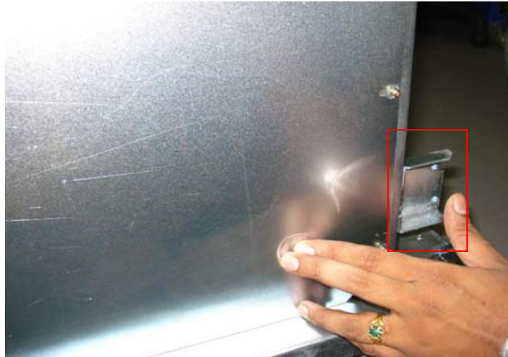
Figure 8-53 Remove LH side EMI cover
