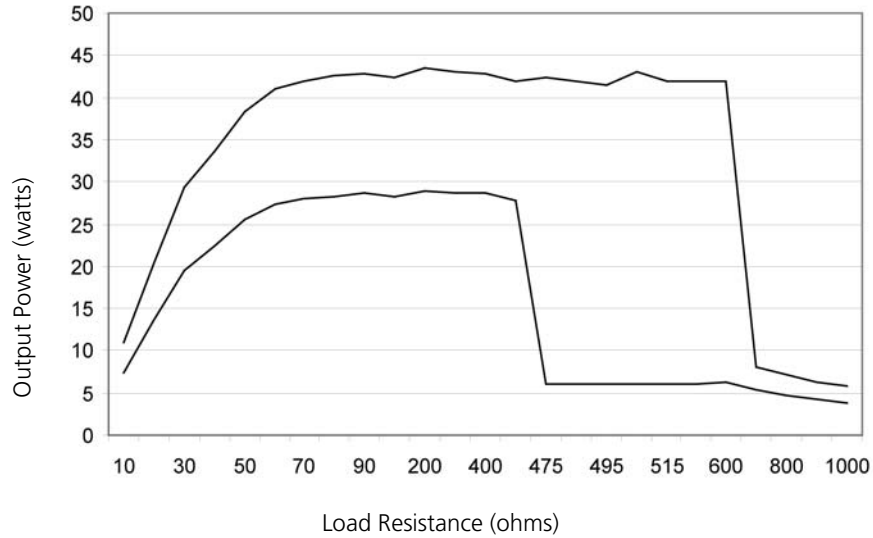
Output power vs. impedance for Standard bipolar 70W mode
