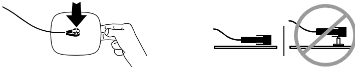
Figure 5-4 Connecting FAST-PATCH Electrodes to Defibrillation Cable
