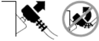
Figure 5-7 Disconnecting Defibrillation Cable from Test Post
